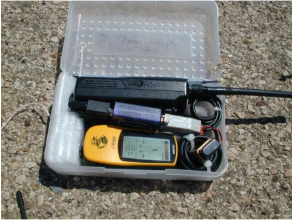
Part 3 - Figure 1. Tracker hardware used during competition. An amateur radio transceiver is located at the top with GPS receiver at bottom. Sandwiched in-between is the TNC. Photo courtesy of David Glover.
